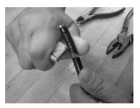
Figure 1 – Ring cut the cable.
