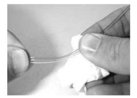
Figure 8 – Clean the optical fibers.
